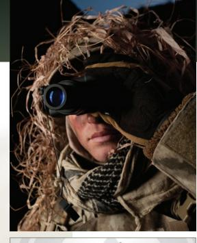
The Armasight Nyx-7 is the bi-ocular night vision goggle built around high grade image intensifier tubes. They are an exceptional choice for hands-free use. Built with high grade optics and simple, reliable electronics, the Nyx-7 provides bright and clear night vision images, even in the most trying conditions. This unit includes a built-in IR light source for reading maps or basic, short-range illumination in complete darkness.
